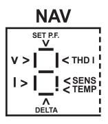
The segment of the NAV display shows the type of measure displayed. Switching on the segment therefore indicates respectively whether the display on the right corresponds to: Voltage, Current, Delta Power, Sensitivity, THD 1%, Set Power Factor, Temperature (the temperature value is showed with the DOT led on).
